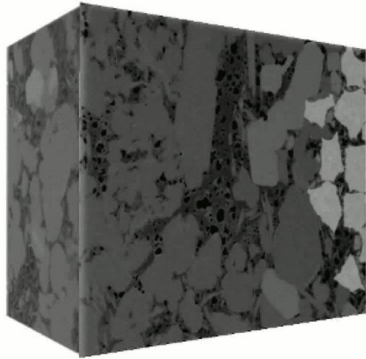
a) A shale micro core sample with size 5\ \mu\text{m} \times 4\ \mu\text{m} \times 3\ \mu\text{m}
