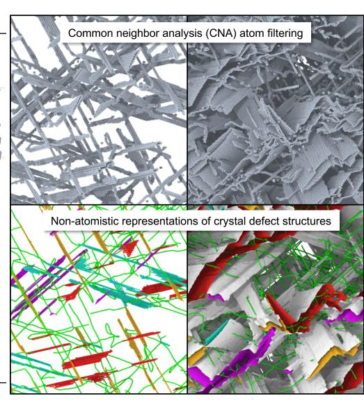
MD simulation of Ta crystal being strained at a
