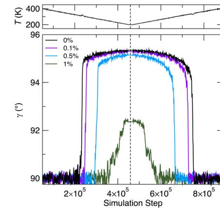
Increasing the concentration of anti-site leads to a more substantial decrease in the phase transformation temperature
