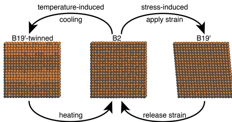
High temperature phase B2 (austenite) has a cubic  $CsCl$ -type crystal structure while the low temperature phase B19' (martensite) is monoclinic.
