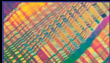
Martensite microstructure in CuAlNi [Bhattacharya 2005]
