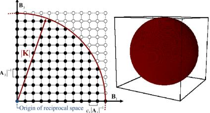
2. Compute diffraction intensities at each point on the reciprocal space mesh using the structure factor equations
